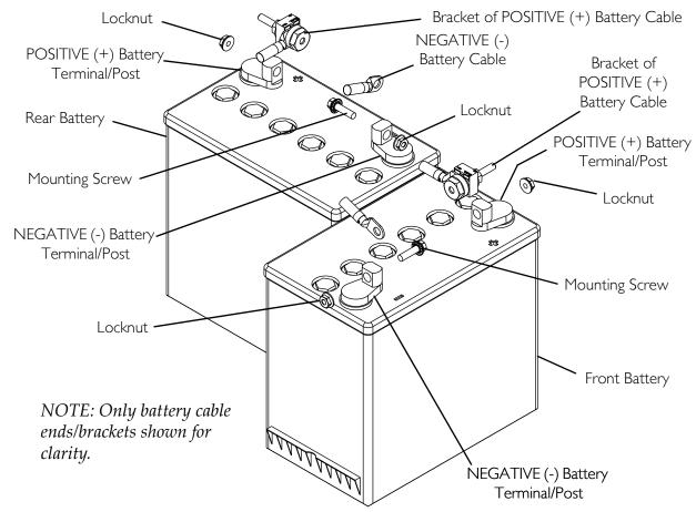
FIGURE 10.1 Replacing Batteries
